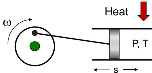
Heating the gas while compressed will raise pressure
