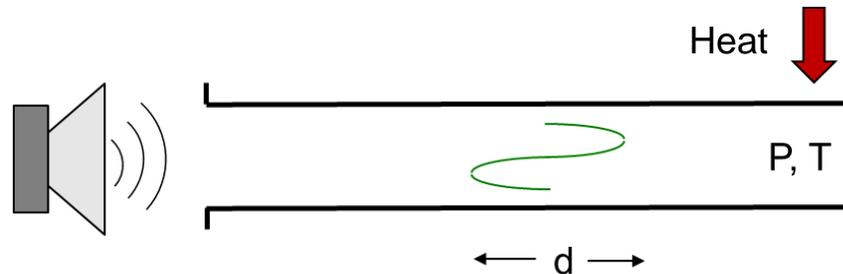
Gas displacement (d) in acoustic waves is similar to piston stroke (s) in mechanical compressors
